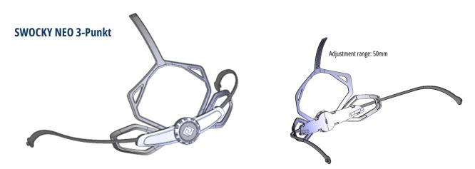
The 3-point version clicks into two side anchoring points in the helmet. A ratchet band on the head cradle, connected to an anchor in the EPS, allows for individual height adjustment, enabling the head cradle to adapt optimally to the head shape.
